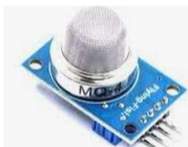
Gambar 2.2 Sensor MQ-4(ShowRange, n.d.)
