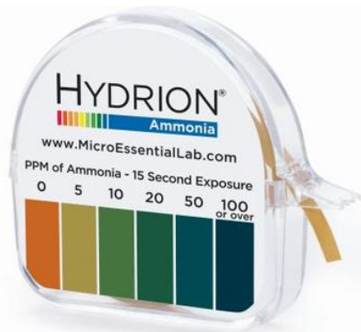
Gambar 2.10. Hydrion AM-40, Ammonia Test Paper (Laboratory, 2020)
