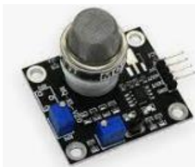
Gambar 2.6 Sensor MQ-137 (ShowRange, n.d.)
