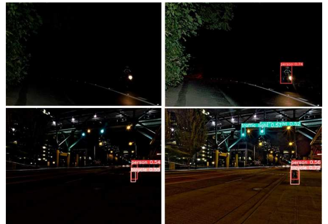
Fig. 5. Example of object detection result using YOLOv5 of original dark image (left) and enhanced image using the proposed approach (right).
